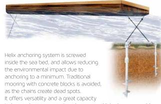
to be used as permanent anchorage, and it is also recoverable. The fastening strength is greater than traditional mooring with concrete blocks or anchors. Even in short anchoring, necessary for overpopulated bays, they keep the fastening strength.
